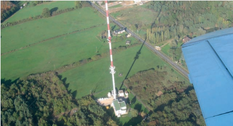
Flux tower set-up for measurements of the greenhouse gas exchange rates over wetland.
