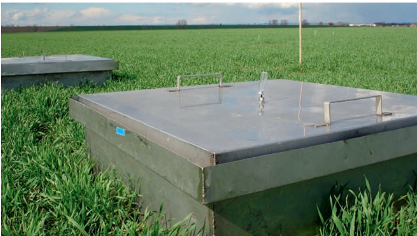
Chamber measurements ( N_2O , CH_4 ) at farmland site, Germany
